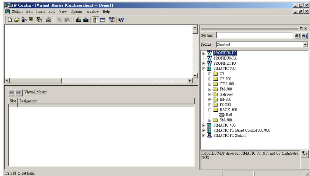
Drag the **Rail** item located under **SIMATIC 300 → RACK-300** (in the hardware catalog window on the right) to the upper half of the **Station** window on the left:
