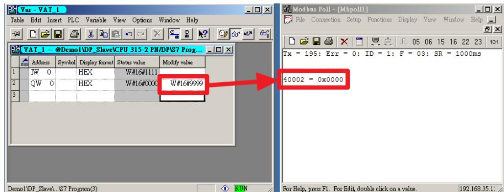
The value of address 40002 is updated by the Output module of the PROFIBUS slave device from 0x0000 to 0x9999.
