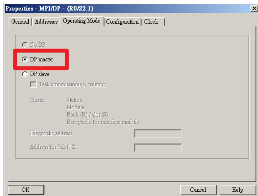
You should then see the results shown in the following figure, indicating that the PROFIBUS network was created successfully.
