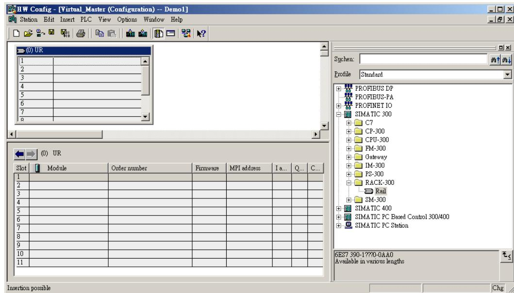
5.2.3. You must add the proper version firmware for the CPU module hardware model. In the figure below, we use **CPU 315-2 PN/DP** as an example. Drag the proper version of the CPU module firmware from the **Hardware Catalog** window on the right and drop it into the empty grid in the **Station** window on the left.
