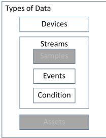
For example, a device named "CNC-1" is composed of a component: DigitalInput:dev\_1. The component then has an Event or Condition data item definition. In this example, the DigitalInput:dev\_1 component has Event data items: "EXECUTION" and "EMERGENCY\_STOP".
