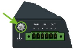
Figure 15: Position of the Grounding Screw
