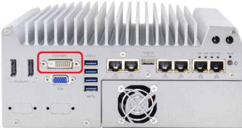
Nuvo-5095GC series has multiple display outputs on its front panel for connecting different displays according to your system configuration. DVI/HDMI transmits graphics data in digital format and therefore can deliver better image quality at high resolution. The DVI/HDMI connector on the front panel can either output DVI signals or HDMI signal depending on the display device connected. It supports up to 1920 x 1200 resolution. You can use a DVI to HDMI cable to connect a HDMI display device.
