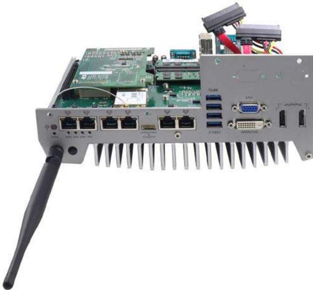
5. Recover the front panel, back panel and the bottom cover and attach a 3G antenna to the SMA connector. The mini-PCle #2 socket shall be used in conjunction with the panel-accessible SIM socket on the back panel. Insert the SIM card upside down to the SIM socket to support 3G communication for your Nuvo-5095GC controller.
