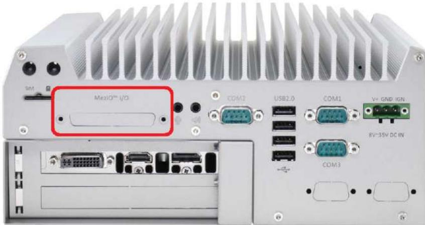
Nuvo-5095GC series incorporates Neusys' MezIO™ interface. You can install a MezIO™ module to expand application-oriented I/O function. To support MezIO™ I/O connectivity, Nuvo-5095GC series reserves the cutting hole for a SCSI-II 68-pin connector on its back panel. Please refer to section 2.5 for information of MezIO™ interface and section 3.6 for installing a MezIO™ module.
