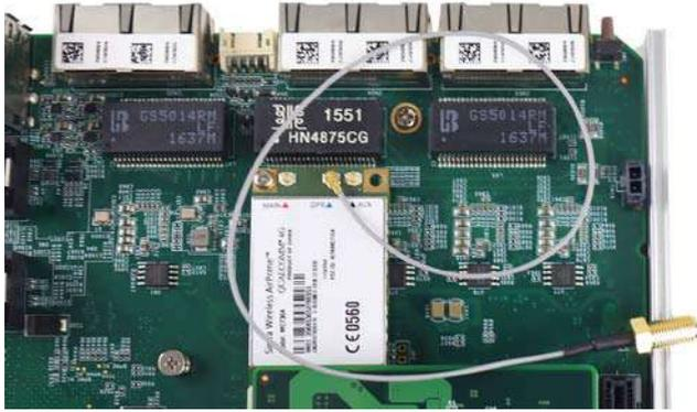
4. Fix the SMA connector of the IPEX-to-SMA cable to one of the four antenna apertures on either front panel or back panel.
