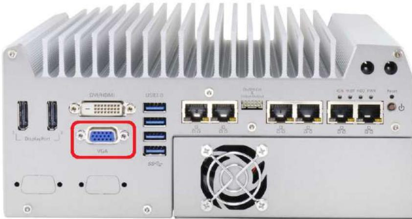
Nuvo-5095GC series has multiple display outputs on its front panel for connecting different displays according to your system configuration. VGA connector is the most popular way for connecting a display. The VGA output on Nuvo-5095GC series supports up to 1920 x 1200 resolution. By BIOS default and hardware implementation, the VGA output is always enabled even when VGA monitor is not connected.
