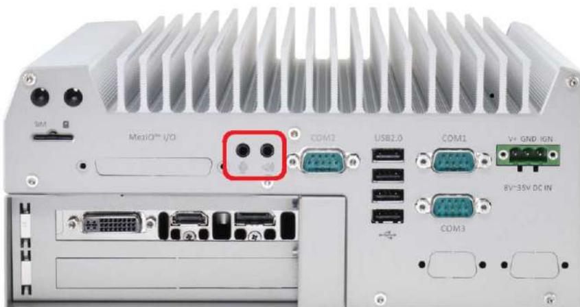
Nuvo-5095GC series provides audio function using Intel® High Definition Audio in Q170 chipset and Realtek ALC262 codec. There are two audio jacks on the back panel. The left one is used for microphone input, and the right one is used for speaker output. To utilize the audio function in Windows, you need to install corresponding drivers for both Intel® Q170 chipset and Realtek ALC262 codec. Please refer to section 4.5 for information of driver installation.
