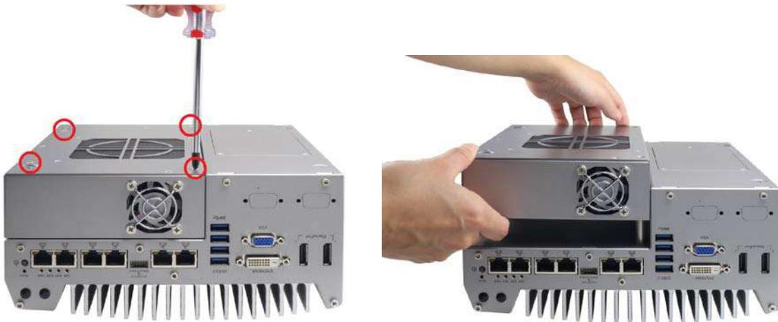
2. Open the cover of Cassette by loosening three M3 flat-head screws.
