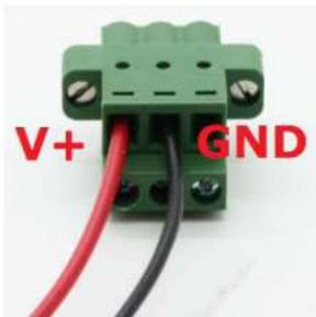
4. Insert the wires to correct contacts of pluggable terminal block and tighten clamping screws using a Philips screwdriver.
