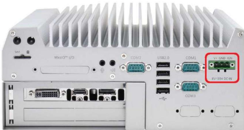
Nuvo-5095GC series allows a wide range of DC power input from 8 to 35V via a 3-pin pluggable terminal block, which is fit for field usage where DC power is usually provided. And the screw clamping connection of the terminal block gives a very reliable way of wiring DC power. For detail information of supplying DC power via pluggable terminal block, please refer to section 3.9.
