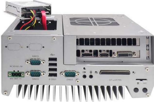
5. Place the HDD/bracket assembly back to the bottom cover. And fix it with three M3 flat-head screws.
