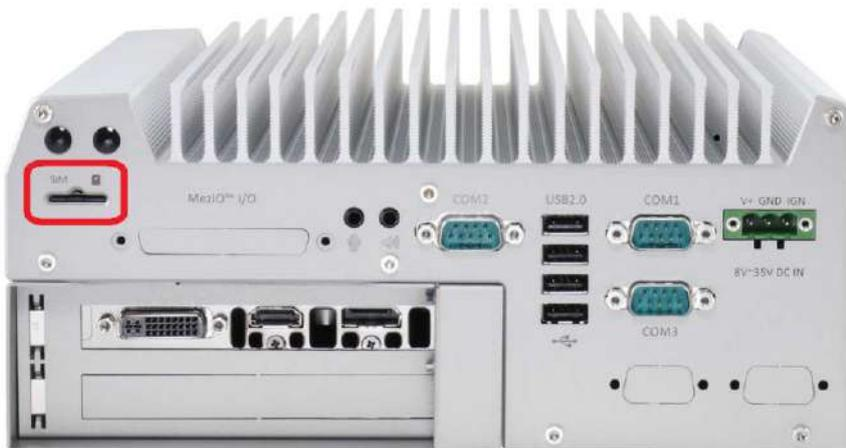
Nuvo-5095GC series provides a panel-accessible SIM socket is on the back panel. Combining with a 3G/4G module installed on internal mini-PCIe port, you can have Internet access via telecom operator's network. The SIM socket is a push-push type. You can insert and push a SIM card to the end to install it, and push the installed SIM card again to eject it. Please note that SIM card must be inserted upside down. You can refer to section 3.5 for information of installing a 3G/4G module and SIM card.
