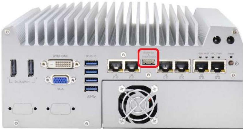
For an application which places Nuvo-5095GC controller inside a cabinet, it's useful to control the on/off of the system via an external switch, as well as check how the system's running via some external LED indicators. Nuvo-5095GC series provides a 2x5, 2.0mm pitch wafer connector on the front panel for this purpose.
