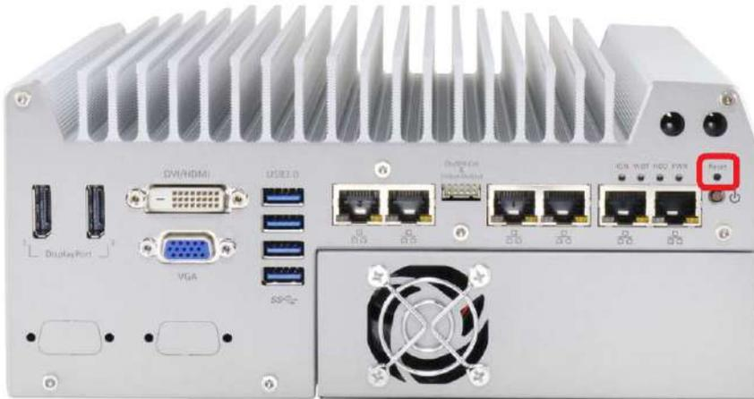
The reset button is used to manually reset the system in case of any abnormal condition. To avoid unexpected operation, the reset button is hidden behind the front panel. You need to use a pin-like object to push the reset button.
