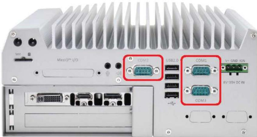
Nuvo-5095GC series provides three COM ports for communicating with external devices. COM1, COM2 and COM3 are located on the back panel via 9-pin D-Sub male connectors. They are implemented using industrial-grade ITE8786 Super IO chip (-40 to 85°C) and provide up to 115200 bps baud rate.
