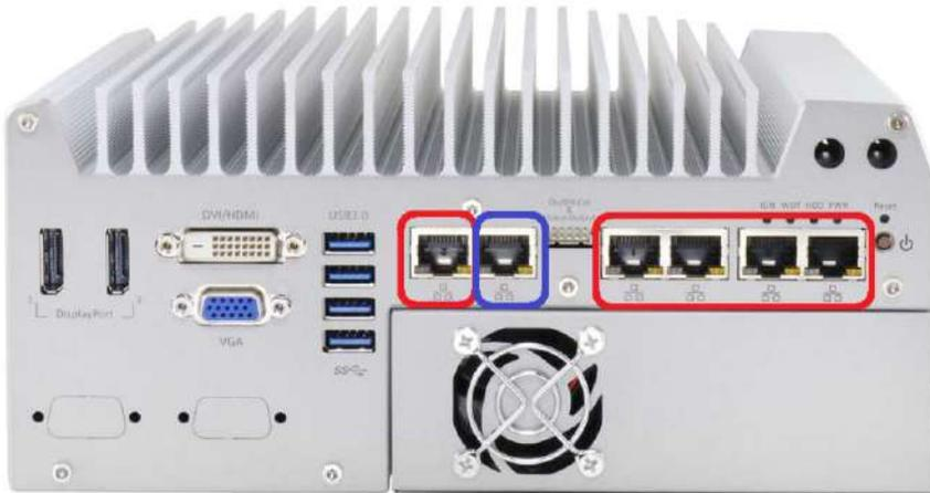
Nuvo-5095GC series offers 6 GbE ports on its front panel. The GbE port marked in blue is designed with Intel® I219-LM and ports marked in red are implemented with Intel® I210-IT Gigabit Ethernet controllers.
