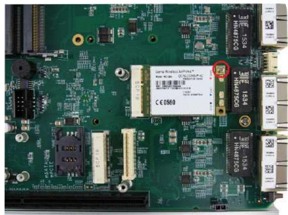
3. Attach the IPEX-to-SMA cable to the 3G module.
