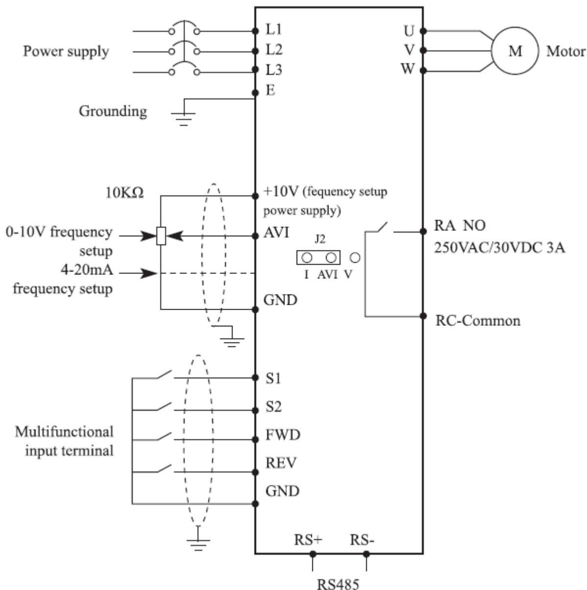
Note: AVI terminals can be used to select an analog voltage input(0-10V) and analog current input (4-20mA ) through the switch J2.
