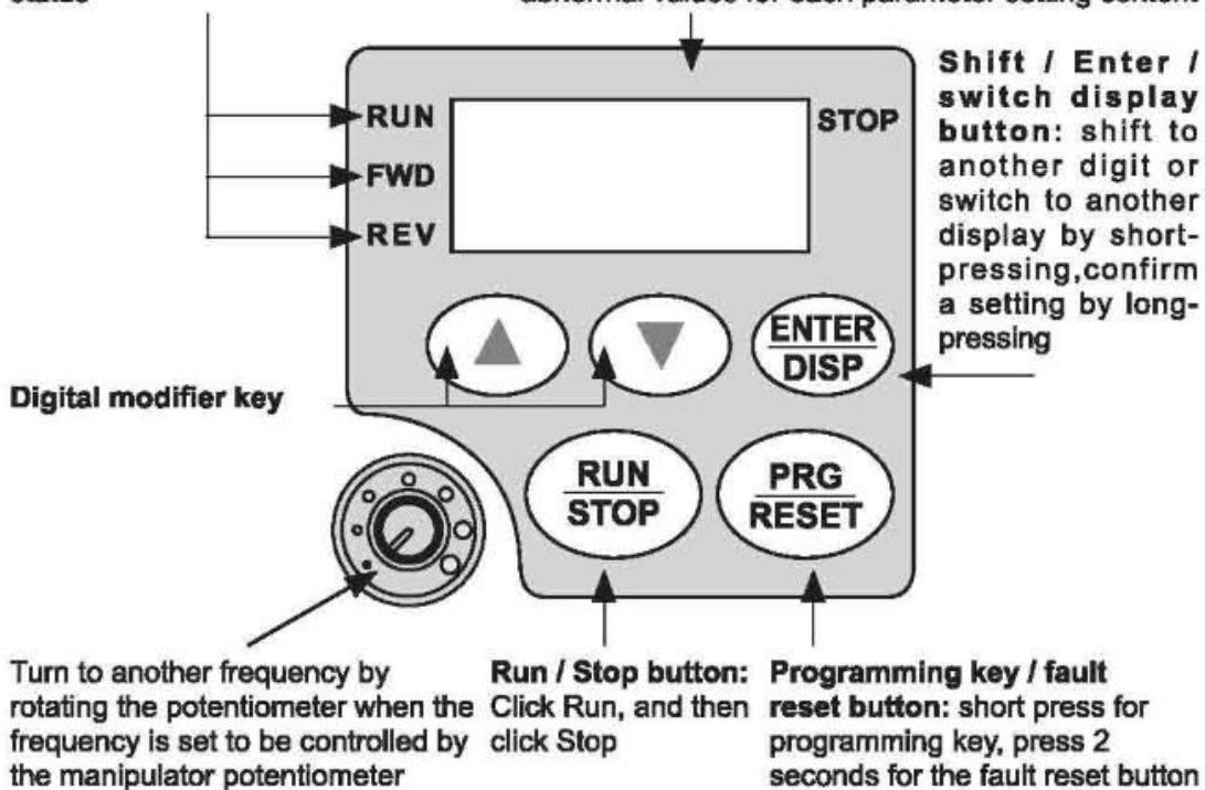
Turn to another frequency by rotating the potentiometer when the frequency is set to be controlled by the manipulator potentiometer
