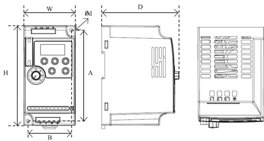
Note: Support for standard 35mm rail mounting(below 5.5kW)
