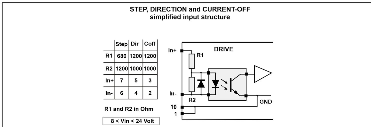
Fig. 1 c: Simplified Input Scheme for A-NDC 96.S
