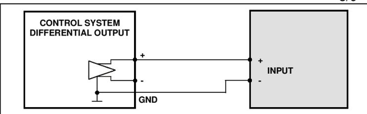
**Fig. 5** Connection example with control system with DIFFERENTIAL output (or LINE DRIVER or RS422).
