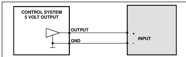
**Fig. 4** Connection example with control system with 5 Volt TOTEM-POLE (PUSH-PULL) output.
