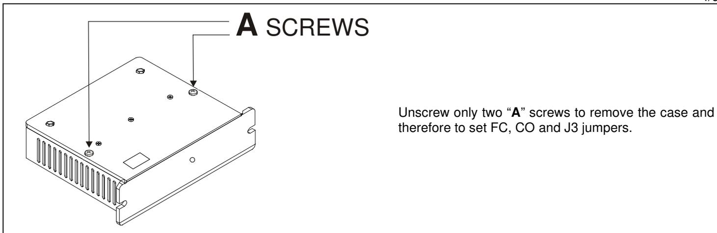
Unscrew only two “A” screws to remove the case and therefore to set FC, CO and J3 jumpers.
