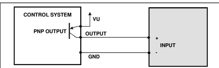
Fig. 3 Connection example with control system with PNP output.
