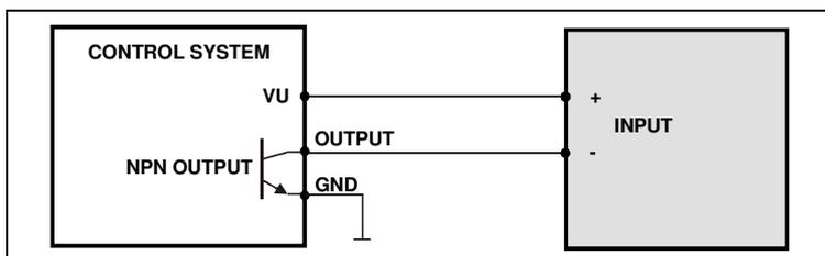
Fig. 2 Connection example with control system with NPN output.
