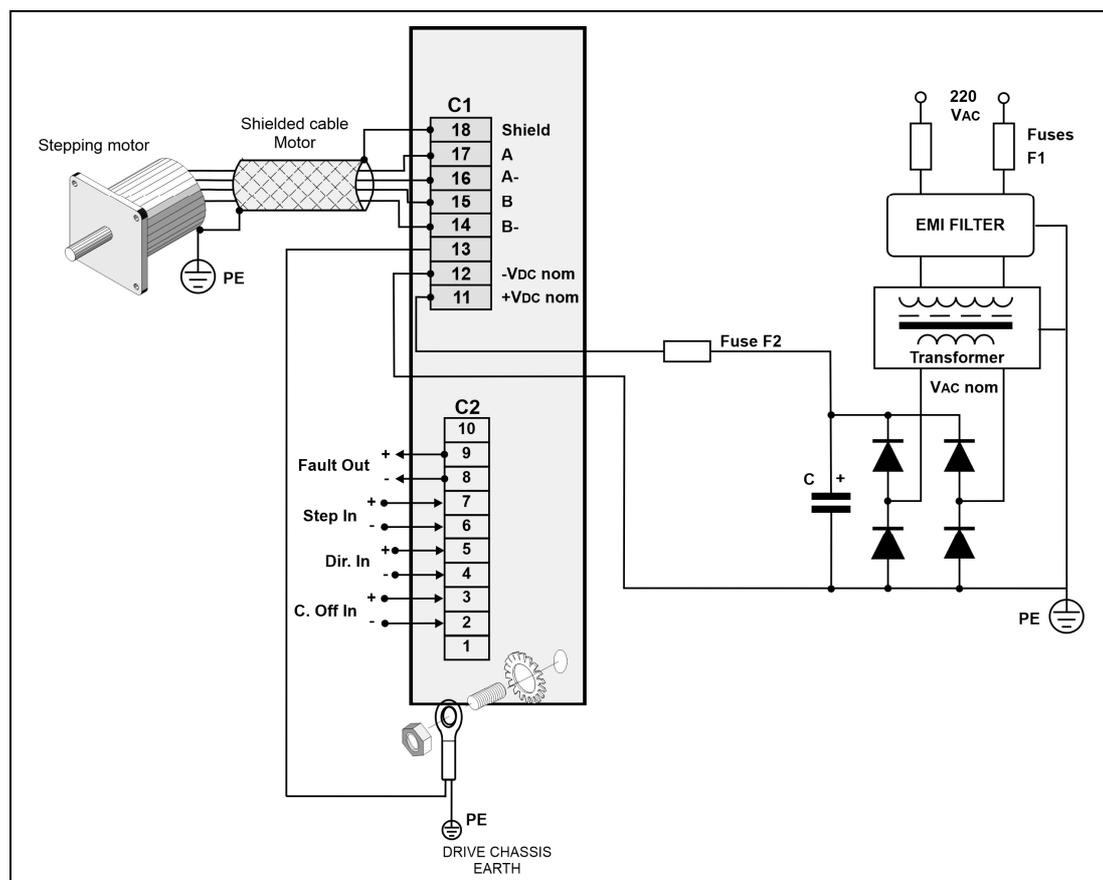
Fig. 7b - Drive external connection scheme for A-NDC 94, A-NDC 96 and A-NDC 96.S.
