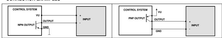
Fig. 2 Connection example with control system with NPN output.
