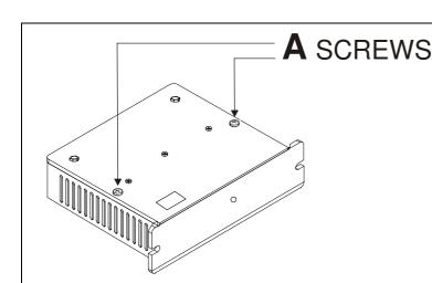
Unscrew only two "A" screws to remove the case and therefore to set FC, CO and J3 jumpers.
