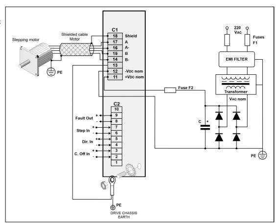
Fig. 7b - Drive external connection scheme for A-NDC 94, A-NDC 96 and A-NDC 96.S.
