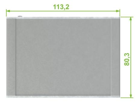
Figure 2: Metal box - Top View
