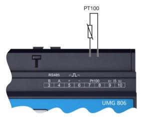
Fig. Connection example for "temperature measurement".
