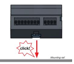
Fig. Mounting on mounting rail
