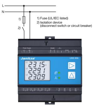
Fig. Supply voltage connection.
