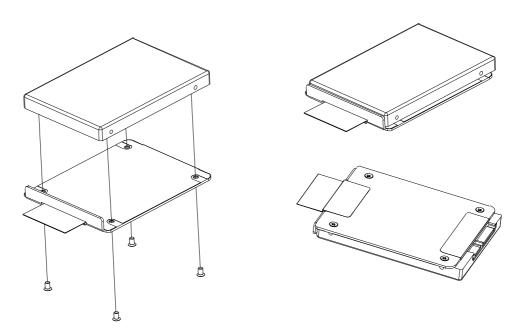
Figure 3.9 SATA HDD Fixed diagram
