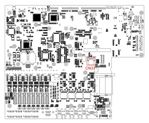
Figure 3.8 CN37 Location of Internal USB Port
