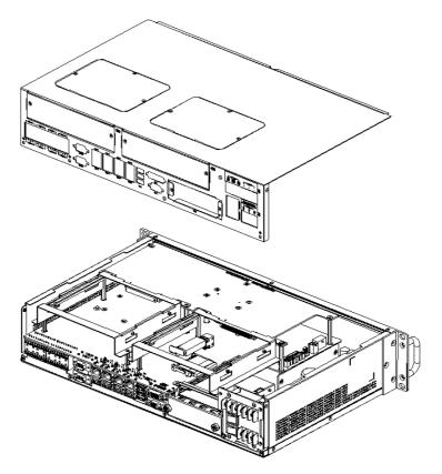
Figure 3.2 ECU-4784 removing top cover
