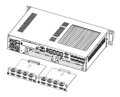
3. Then secure the expansion cards using the previously removed screws.
