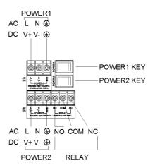
Figure 2.5 Power1&Power 2 input location
