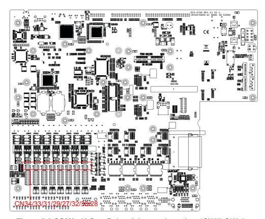
Figure 2.9 COM3~10 Port Related Jumper Locations(CN27-CN34)
