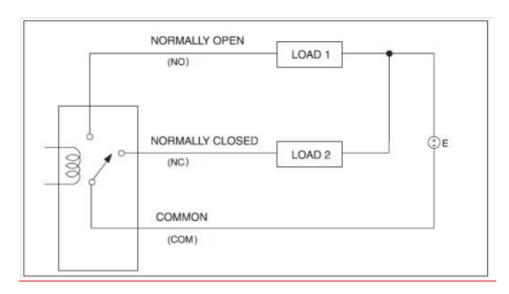
Figure 2.11 Wiring Diagram of the Relay Out
