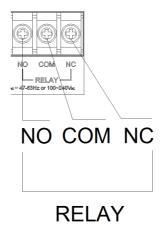
Figure 2.10 Relay output connections
