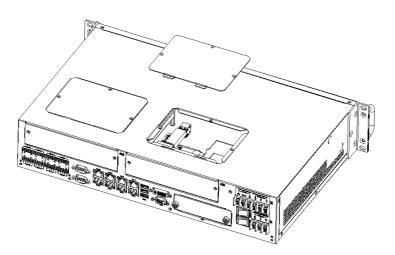
Figure 3.6 Open the chassis
