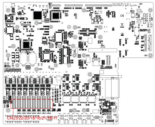
Figure 2.7 COM3~10 Port Related Jumper Locations (CN16-CN23)
