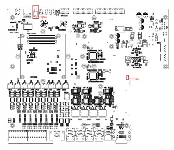
Figure 2.6 AT X /AT Power Mode Select location (CN60)
