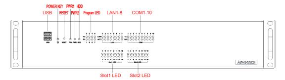
Figure 2.1 ECU-4784 Front Panel
