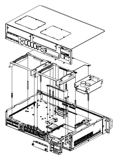
Figure 1.3 ECU-4784 Series Explode picture
