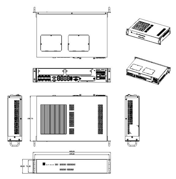
Figure 1.2 ECU-4784 Series Chassis Dimensions
