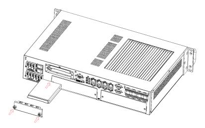
Figure 3.10 HDD back plate location and SATA HDD Installation diagram
