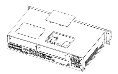
Figure 3.4 CFast Card Slot Location (CN3)
