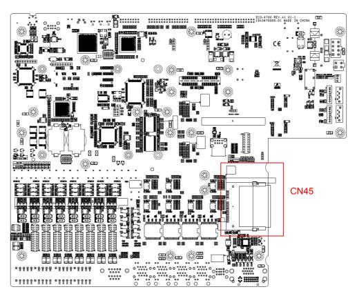
Figure 3.5 CFast Card Slot Location (CN45)
