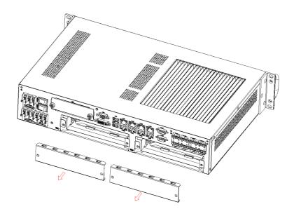
2. Plug in the PCI Card or PCIE Card through the DIN-Rails.
