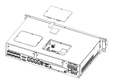
Figure 3.7 CN14 Location of Internal USB Port
