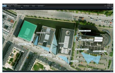
The map function is an interactive operational security hub providing operators situational overview and instant access to cameras and other security peripherals
