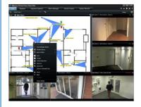
It is also possible to remotely open/close and lock/unlock access points via the map.
