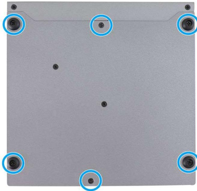
2. Gently lift the bottom panel of the enclosure and remove the screws indicated.
