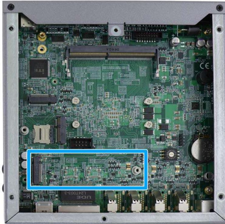
2. Insert the module on a 45 degree angle.
