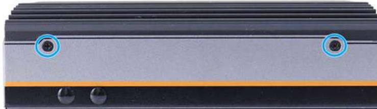
**Right side chassis screws securing the heatsink**
