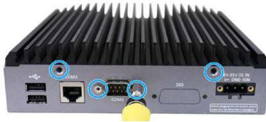
**Remove screws on I/O panel**
