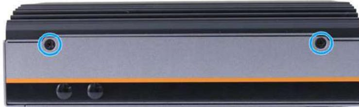
**Left side chassis screws securing the heatsink**
