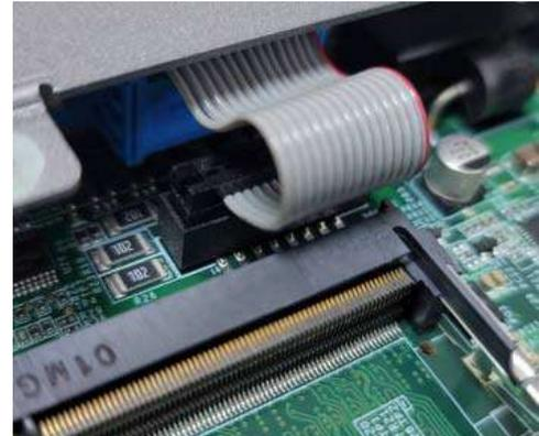
**Match the connector to the DIO port    Make sure the connector is properly inserted**
