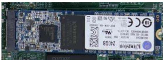
3. Gently press down and secure the module with an M3 P-head screw.
