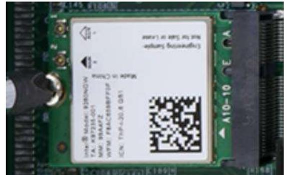
Secure using the screw provided
