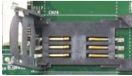
Slide and lift SIM card holder
