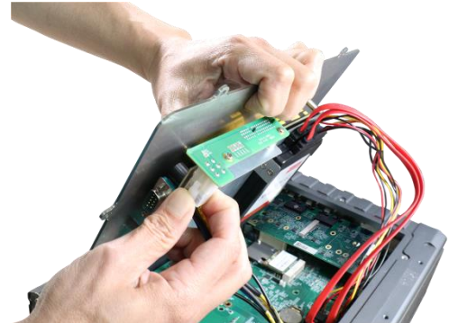
Plug in the 4-pin ATX connector
