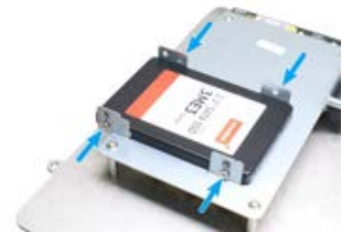
Secure hard drive with screws on both sides
