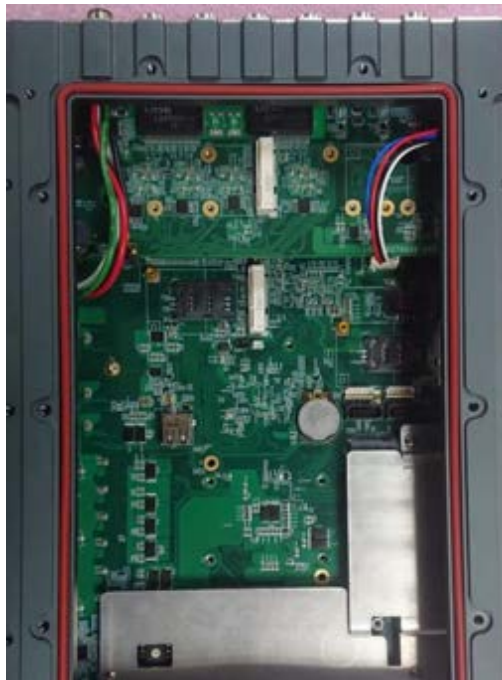
O-ring seated properly in the groove
