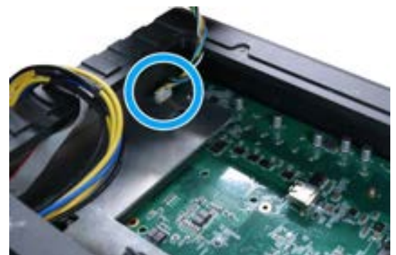
Unplug the 4-pin ATX connector
