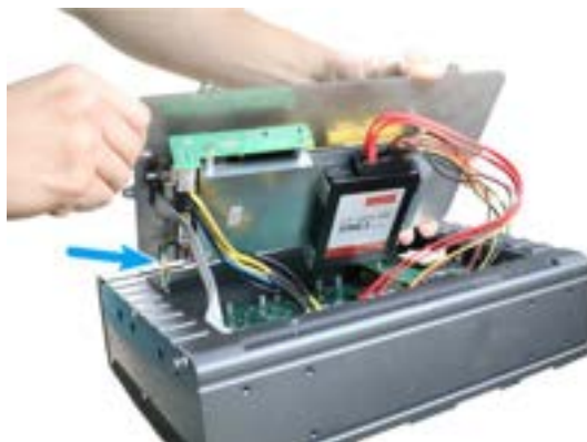
Disconnect the 4-pin power connector
