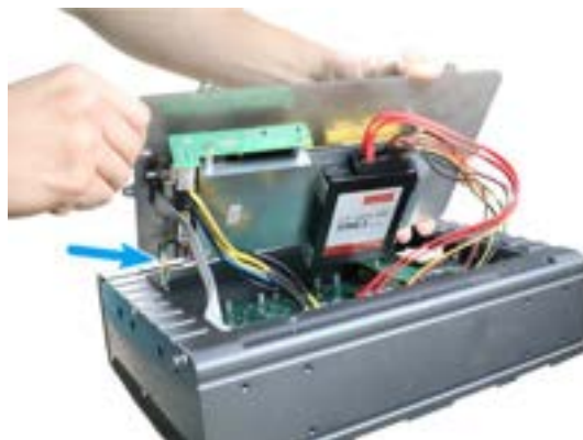
Disconnect the 4-pin power connector
