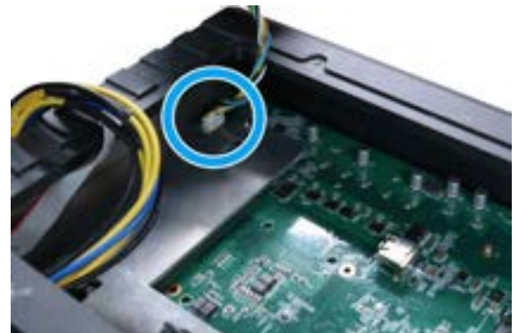
Unplug the 4-pin ATX connector
