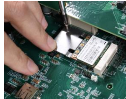
Secure the module with a screw
