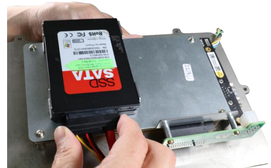
Then connect the hard drive on top (if installed)
