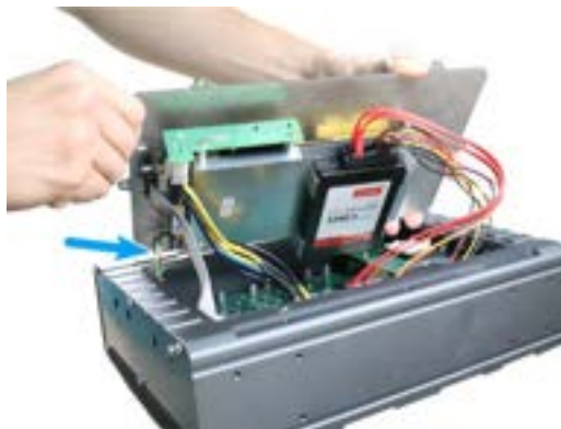
Connect the 4-pin power connector
