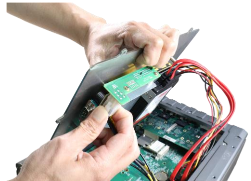
Unplug the 4-pin ATX connector
