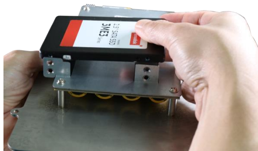
Place hard drive in between brackets
