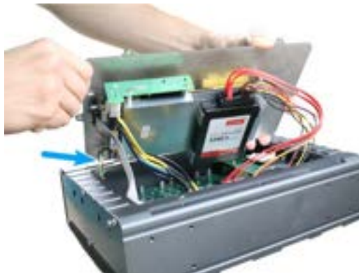
Connect the 4-pin power connector
