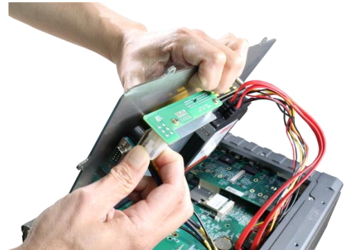
Plug in the 4-pin ATX connector
