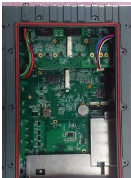
O-ring seated properly in the groove
