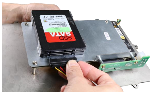
Connect the bottom hard drive first
