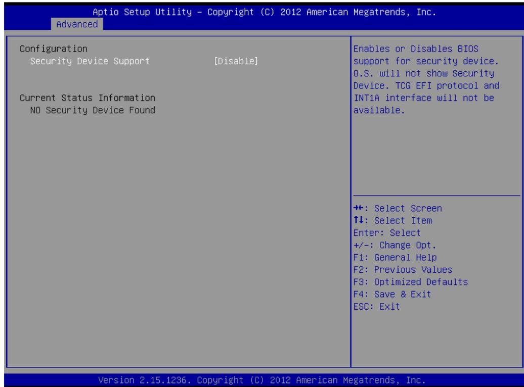
**Figure 5.7 Trusted Computing Configuration**
