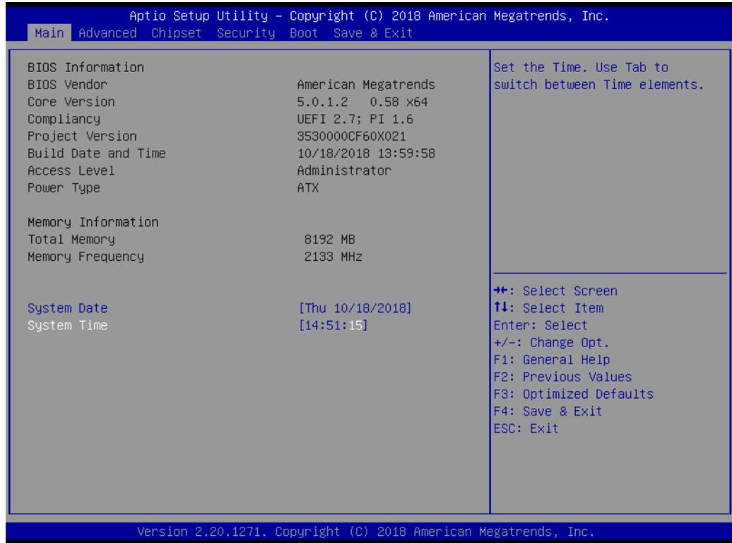
AMI's BIOS ROM has a built-in Setup program that allows users to modify the basic system configuration. This information is stored in flash ROM so it retains the Setup information when the power is turned off.
