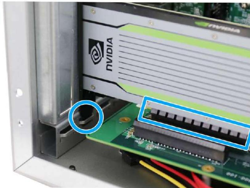
5. Secure the inference accelerator's bezel.
