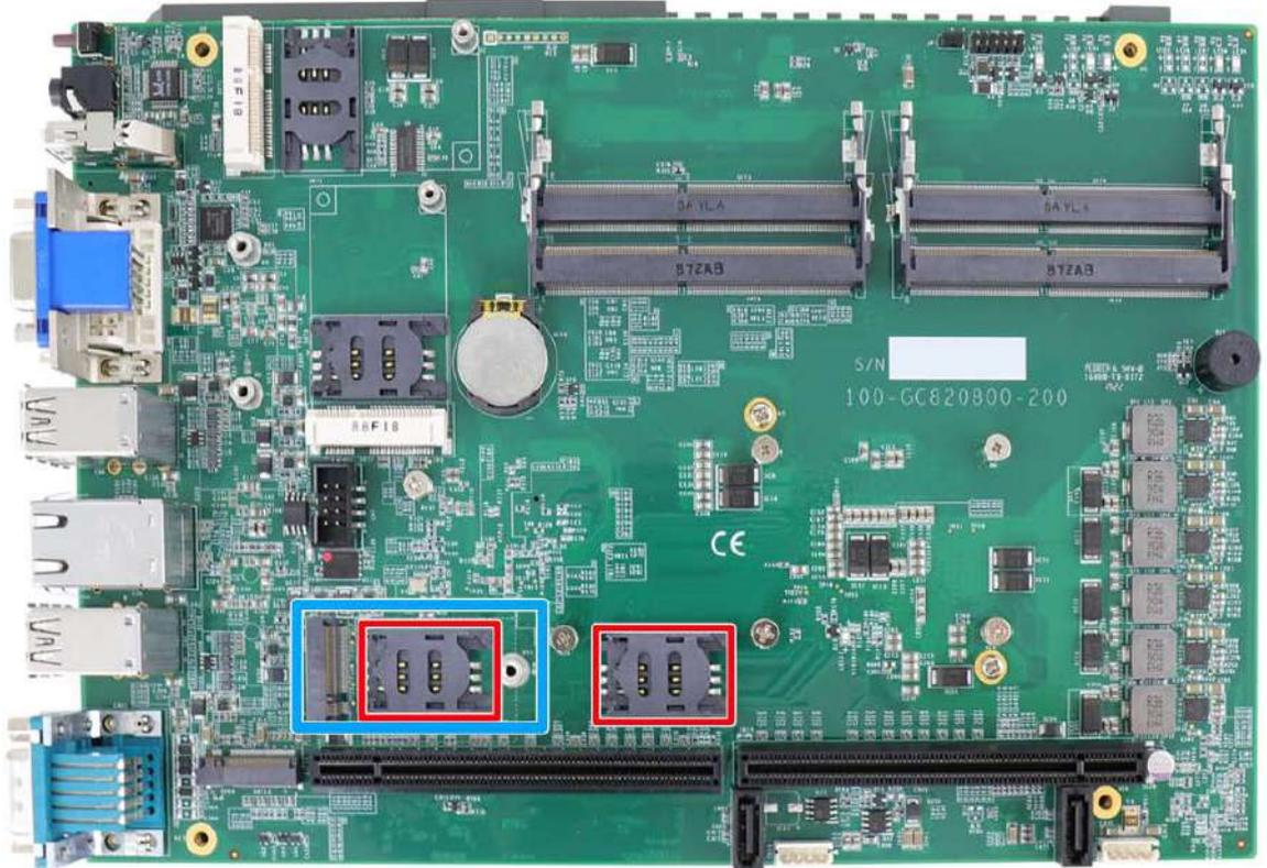
The system has an M.2 2242 slot (indicated in **blue**) that works with dual SIM slots (4G + 3G) on the front panel (indicated in **red**). By installing a 3G or 4G M.2 module and SIM card, you can access the internet via the provider's network.
