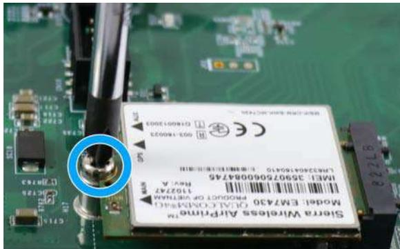
7. Clip on the IPEZ-to-SMA cable to the module and secure the antenna connector body to the panel and install the antenna. Please refer to the module's manual for clip-on connection.
