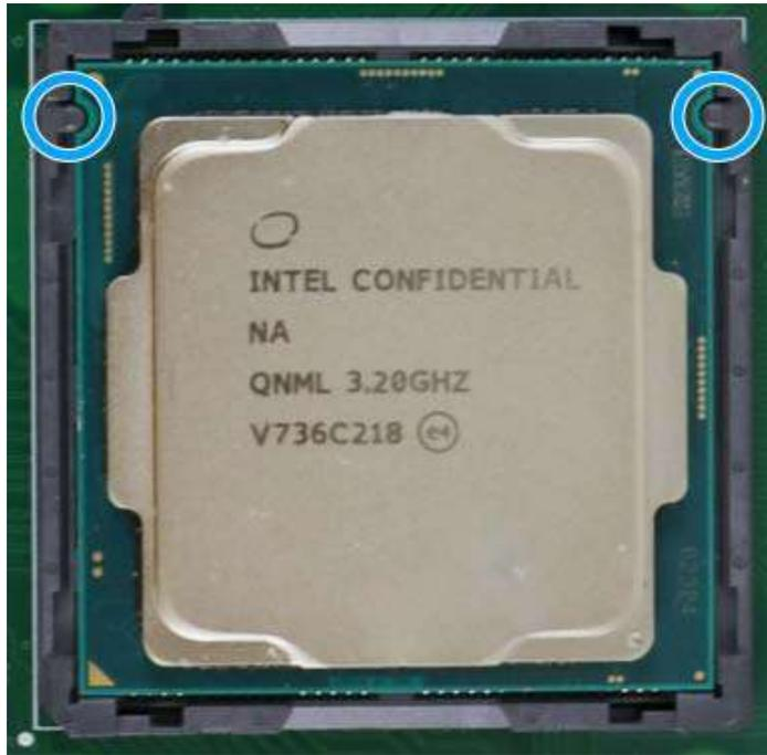
6. Locate the CPU retention bracket from the accessory box. Place the retention bracket on the CPU and hold it in place.
