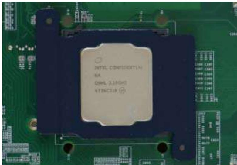
7. Turn the motherboard around and secure the bracket by tightening two M3 P-head screws.
