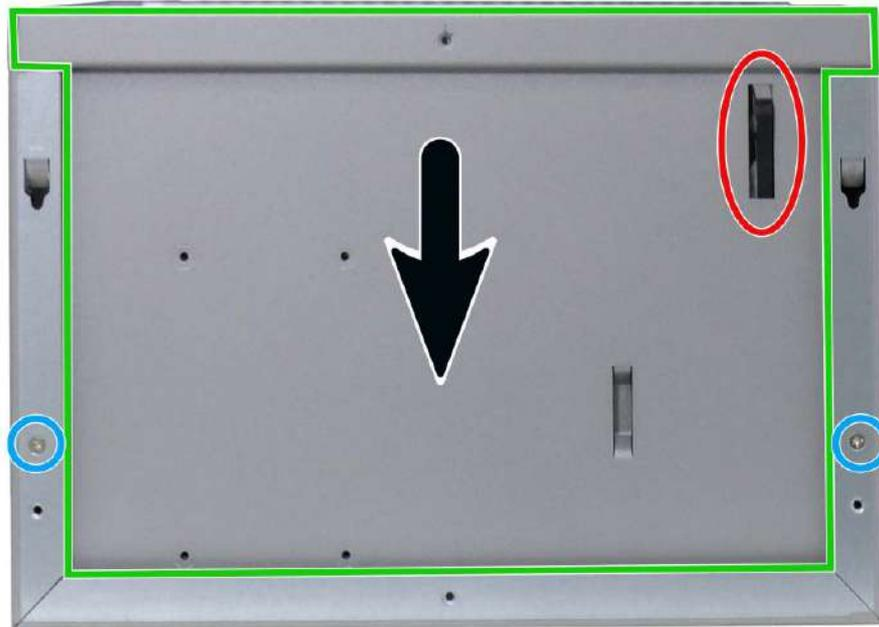
2. Holding the L-shape panel by the handle at the top, lower the L-shaped panel onto the enclosure.
