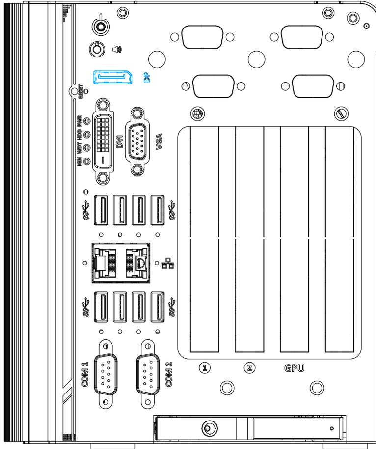
The DisplayPort (DP) output is a digital display interface that mainly connect video source and carry audio to a display device. When connecting a DP, it can deliver up to 4K UHD (4096 x 2304) in resolution. The system is designed to support passive DP adapter/ cable. You can connect to other display devices using DP-to-HDMI cable or DP-to-DVI cable.
