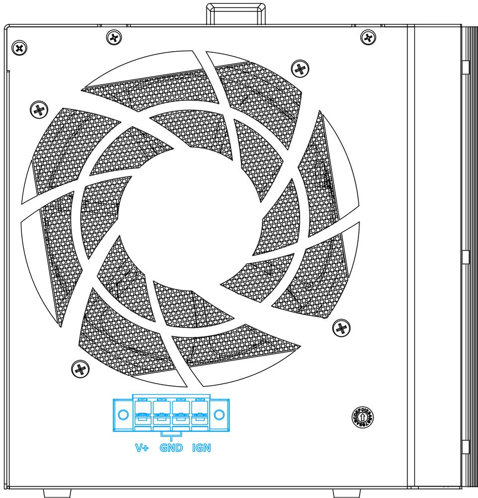
The system accepts a wide range of DC power input from 8 to 48V via a 4-pin pluggable terminal block, which is fit for field usage where DC power is provided. The screw clamping mechanism on the terminal block offers connection reliability when wiring DC power. In addition to DC power input, this terminal block can also accept ignition signal input (IGN) for in-vehicle applications.
