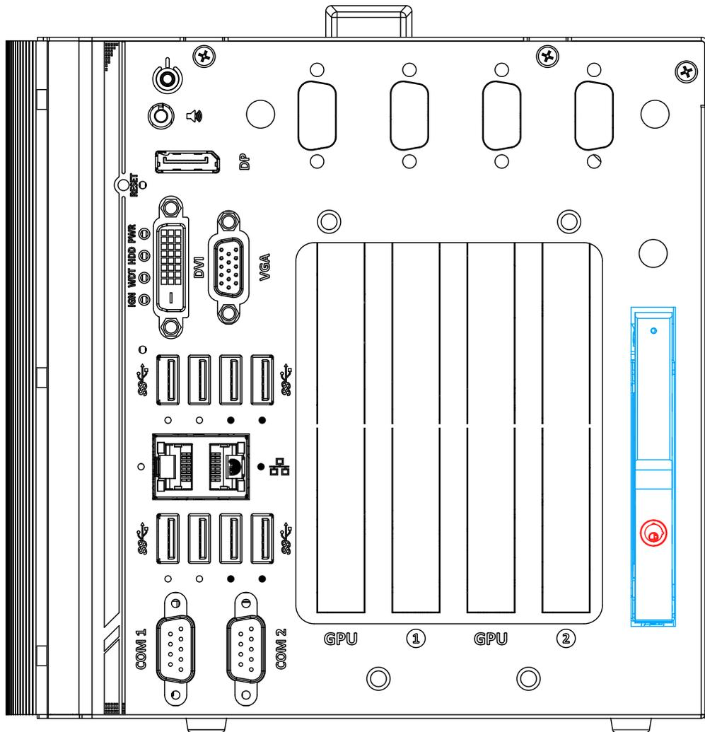
The system has an external 2.5” HDD/ SSD via a hot-swappable tray. Designed for easy access, the HDD/ SSD slot is secured by a lock (indicated in **red**) and it supports RAID modes 0/ 1 configuration by combining with the internal HDD/ SSD drive for OS installation (coupled with the internal HDD). To set up RAID, please refer to RAID Volume Configuration section for details.
