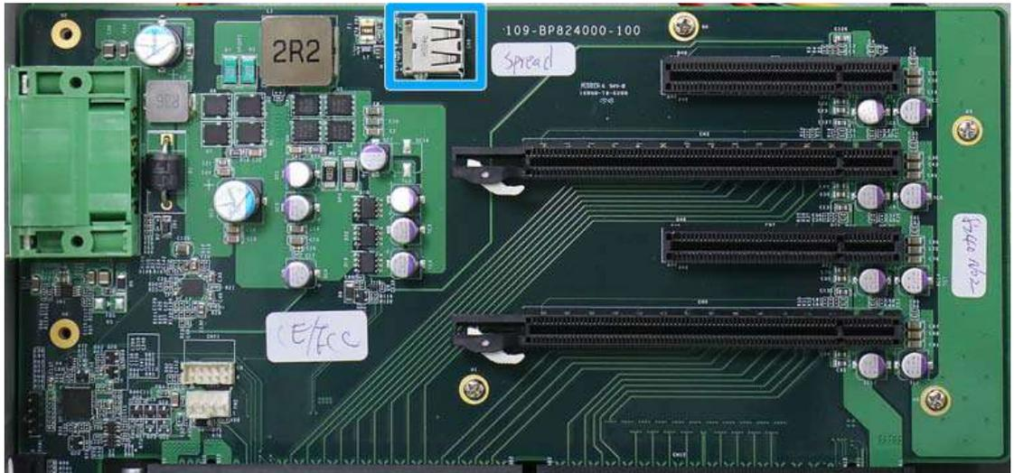
The system's daughter board has an internal USB2.0 port on the PCBA. You can utilize this USB port to connect a USB protection dongle inside the chassis of the system.
