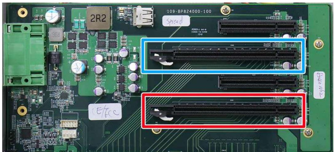
3. Remove the corresponding enclosure bezel(s) to the PCIe slot you wish to install to .
