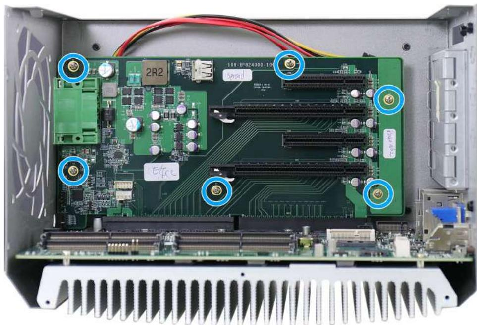
7. Gently pull and slide the extension board out of the enclosure to gain access to internal expansion slots.
