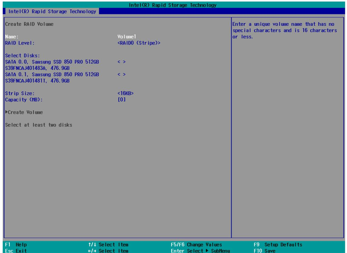
9. The RAID Level option allows you to select RAID-0 (striping) or RAID-1 (mirror) for your RAID volume. Press ENTER when ready.
