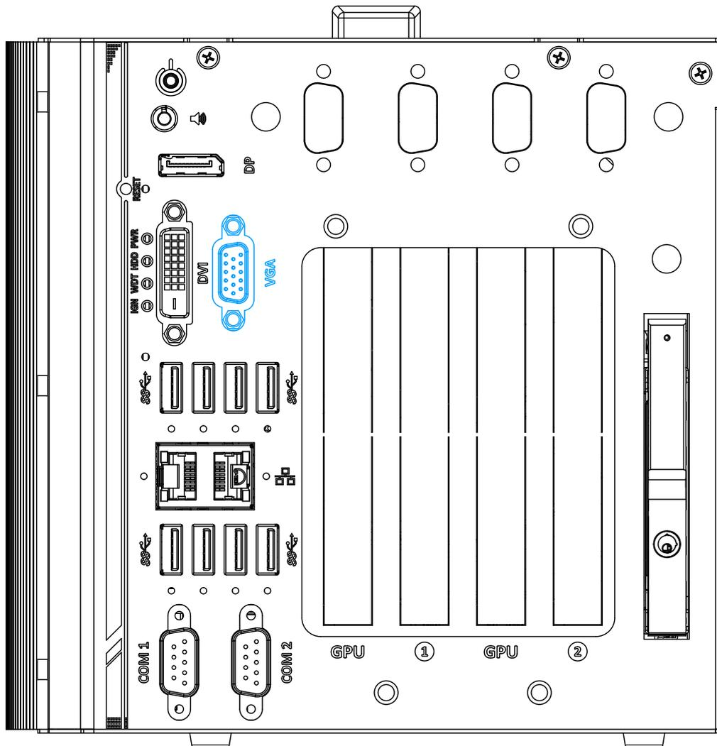
VGA connector is the most common video display connection. The VGA output supports up to 1920x1200@60Hz resolution.
