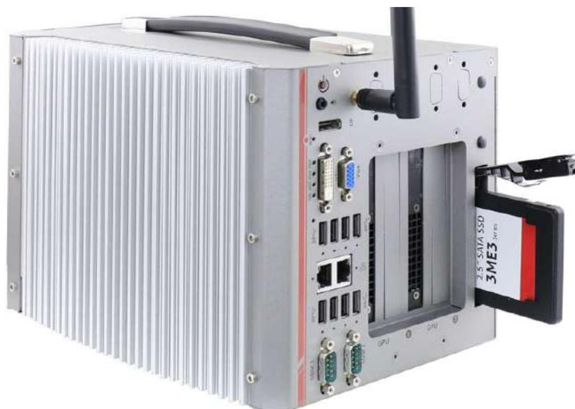
3. Push the handle into the 2.5" slot until it snaps into position. A key is provided (in accessory box) to lock the external slot.
