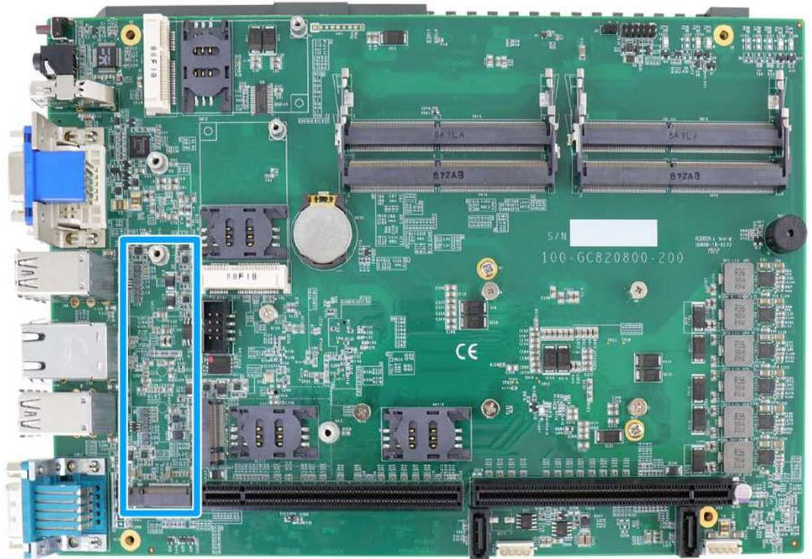
The system has an x4 PCIe M.2 2280 slot (also in compliance with SATA signal) for you to install an NVMe SSD for the ultimate performance or an Intel® Optane™ memory to accelerate the read/ write performances of traditional hard disk drive. An NVMe SSD offers exceptional performance over 2.5" SSDs while Intel® Optane™ memory can dramatically boost your traditional hard disk drives' read/ write performances.
