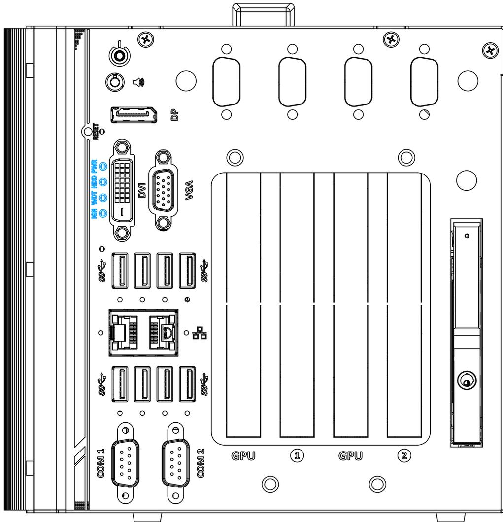
There are four LED indicators on the I/O panel: PWR, HDD, WDT and IGN. The descriptions of these four LED are listed in the following table.
