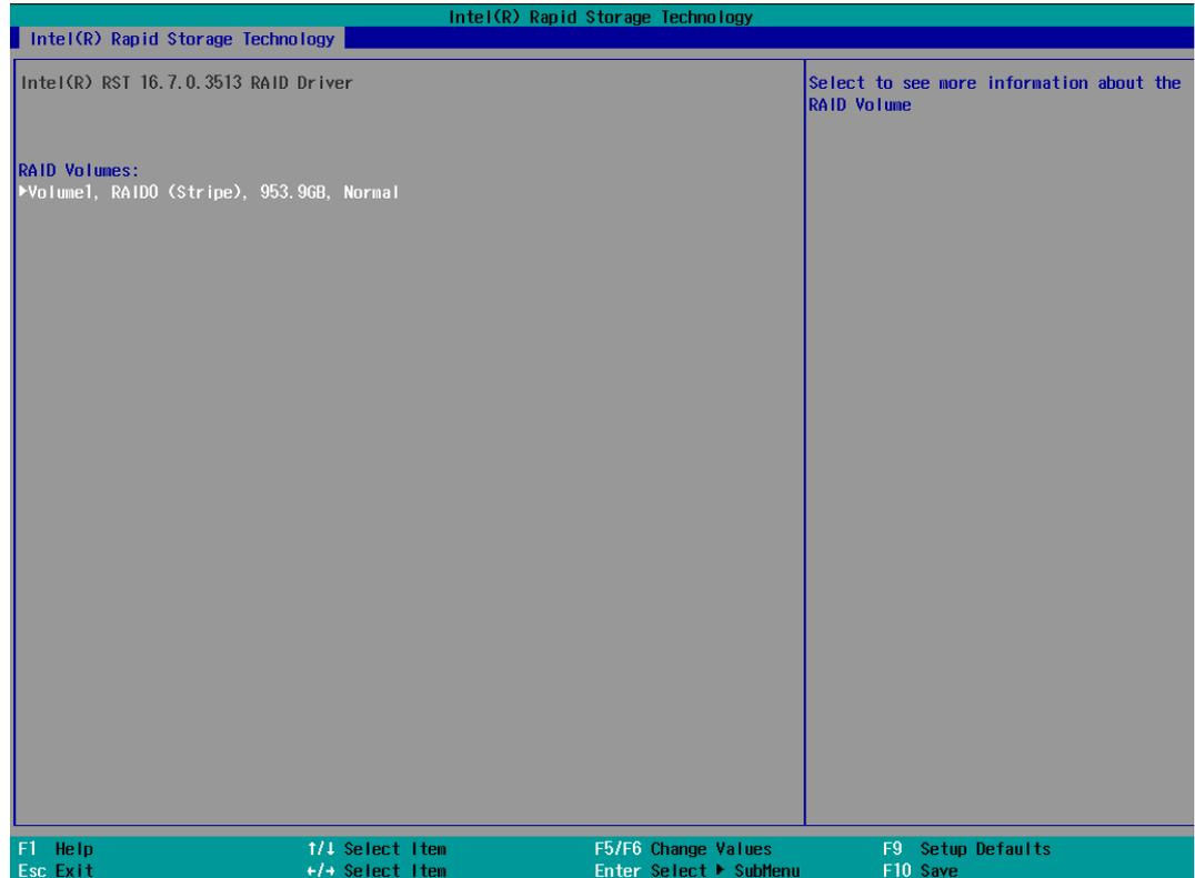
15. Press F10 to save and Esc to exit the Intel® Rapid Storage Technology configuration page.
