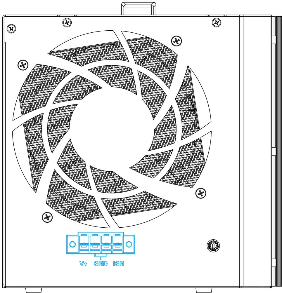
To have ignition power control for in-vehicle usage, you need to supply IGN signal to the system. The IGN input is located on the 4-pin pluggable terminal block (shared with DC power input). Below is the typical wiring configuration for in-vehicle applications.
