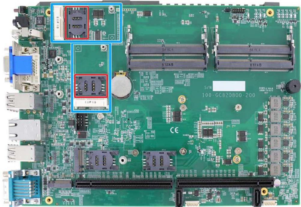
3. Before installing the mPCIe module, you need to insert the Mini-SIM card. Slide the SIM slot holder and lift the SIM card holder. Insert the Mini-SIM card (pins facing up), shut the SIM holder and slide it to lock the SIM card in-place.
