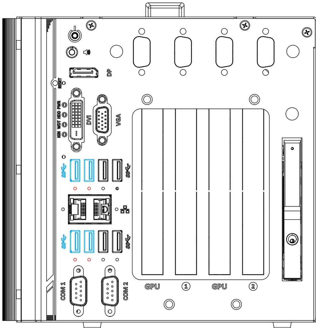
The system's USB 3.1 Gen 2 ports (10Gbps) are implemented via native xHCI (eXtensible Host Controller Interface) controller and are backward compatible with USB3.1 Gen.1 USB 2.0, USB 1.1 and USB 1.0 devices. Legacy USB is also supported so you can use USB keyboard/mouse in DOS environment. There are also screw-lock openings (indicated in **red**) for each USB port.
