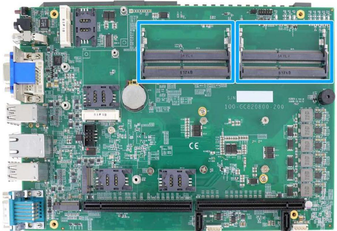
The system motherboard supports four 260-pin SODIMM socket for installing DDR4 memory module up to 128GB. Each slot supports single module DDR4 2133MHz SODIMM up to 32GB capacity.
