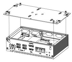
2. Unscrew the blacking plate screws to remove the blanking plate.
