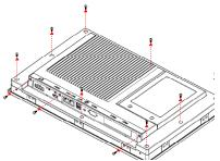
2. Unscrew the blacking plate screws and remove the blanking plate.
