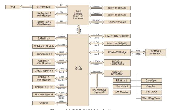
Figure 1.3 PCE-5129 block diagram
