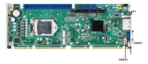
Two on-board 6-pin mini-DIN connectors (KBMS1) provide connection to a PS/2 keyboard and mouse via the Y-cable (1700060202) in the package.
