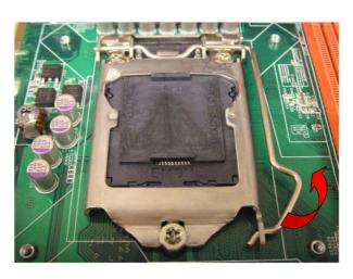
2. Remove the socket protection cap.
