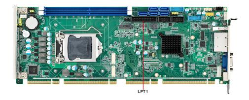
The parallel port is normally used to connect the motherboard to a printer. The SBC includes an onboard parallel port, accessed through a 26-pin flat-cable connector.
