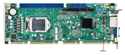
LPC1 is a 14-pin female pin header for connection with an Advantech LPC module.
