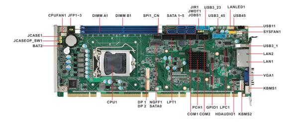
Figure 1.1 Jumper and connector locations
