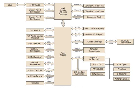
Figure 1.2 PCE-7129 block diagram
