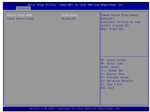
**Figure 3.10 Secure Erase Configuration**
