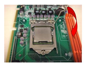
5. The finished processor installation.
