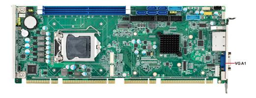
This CPU card has a VGA output that can drive a conventional CRT display. VGA1 is a standard 15-pin D-SUB connector commonly used for VGA.
