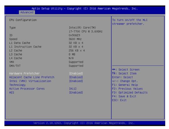
Figure 3.5 CPU Configuration
