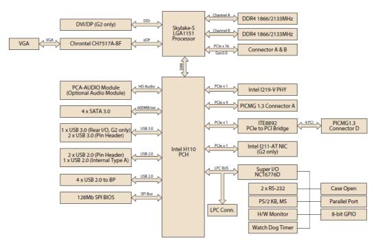
Figure 1.4 PCE-5029 block diagram
