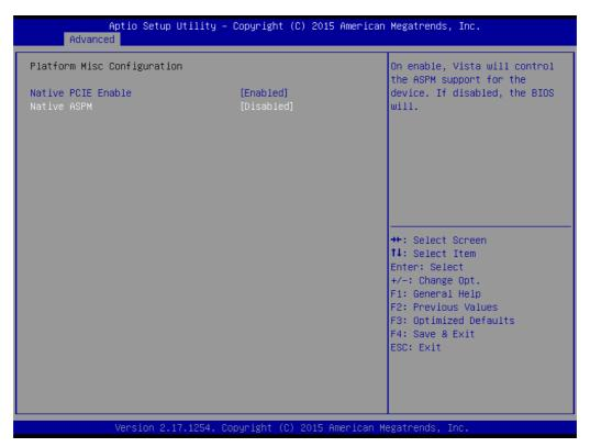
**Figure 3.4 Platform Misc Configuration**
