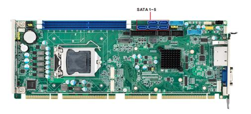
The PCE-7129/5129/5029 features high performance serial ATA interface (5\*600MB/ s) which eases cabling to hard drivers or CD/DVD drivers with long cables. These five on-board SATA ports can be configured as RAID 0, 1, 10, or 5(PCE-5029 do not support RAID). Please see the detailed BIOS setting instructions for this in Chapter 3.
