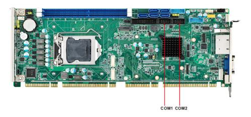
These SBCs offer two serial ports. These ports can connect to serial devices, such as a mouse or a printer, or to a communications network.
