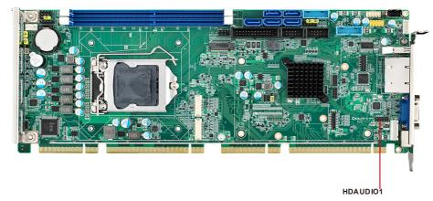
This HDAUD1 pin header is the connection interface to Advantech's high definition audio module.
