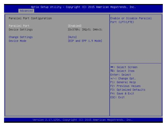
**Figure 3.19 Parallel Configuration**
