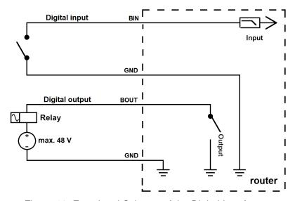
Figure 18: Functional Scheme of the Digital Interface
