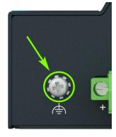
Figure 16: Position of the Grounding Screw
