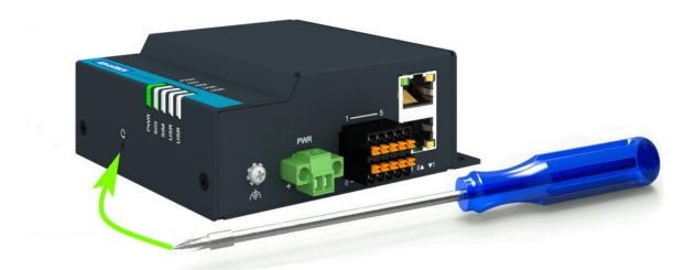
Figure 20: Resetting the Router
