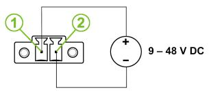
Figure 15: Power Connector Pinout
