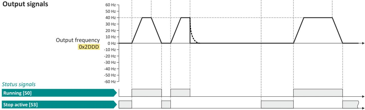
The status signals can be assigned to digital outputs. [▶ Configure digital outputs](#) 292
