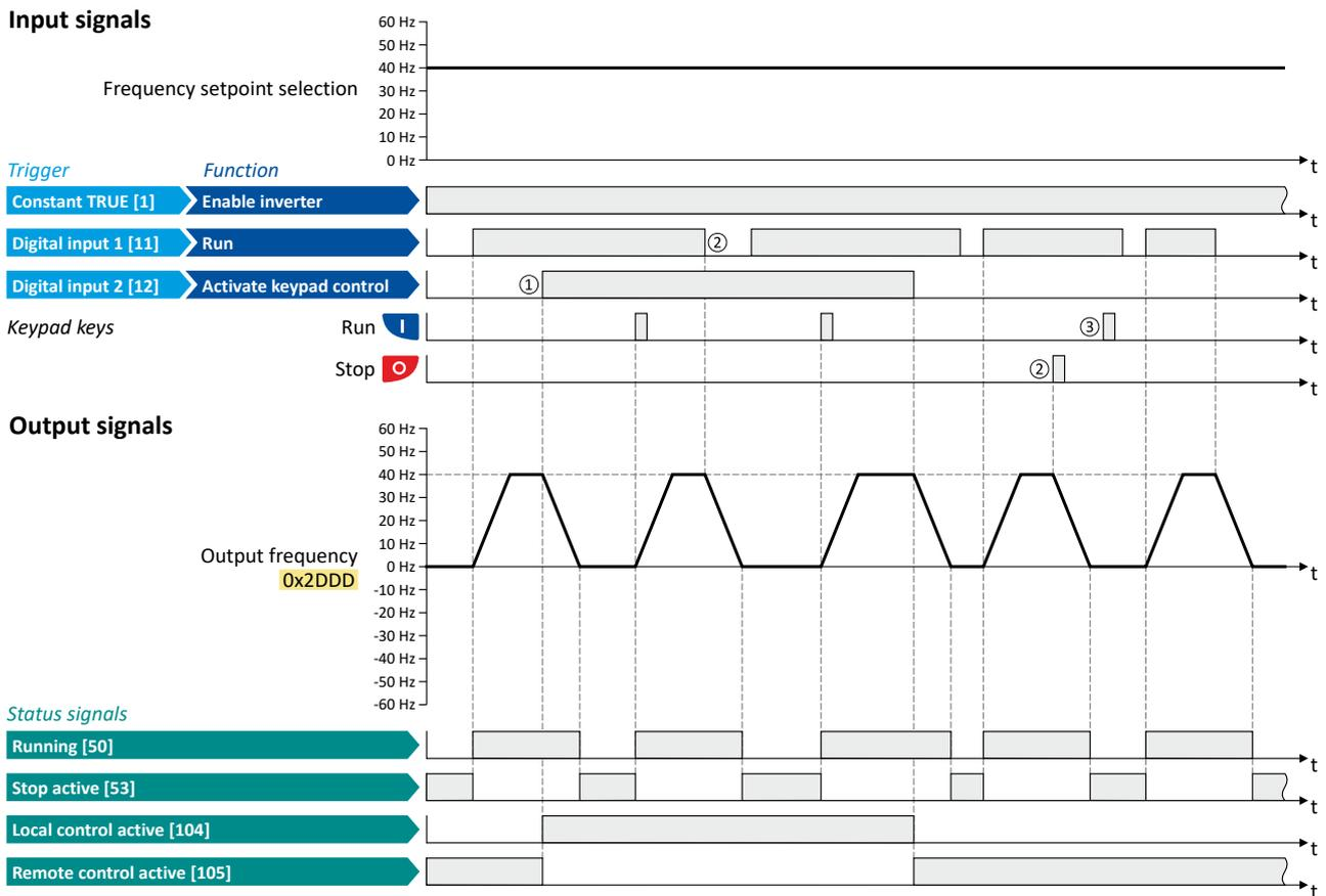
The status signals can be assigned to digital outputs. ▶ [Configure digital outputs](#) 292
