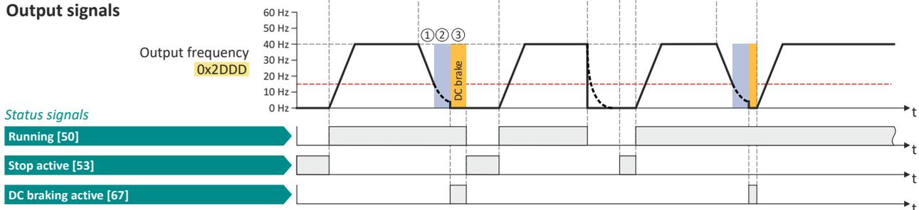
The status signals can be assigned to digital outputs. ▶ [Configure digital outputs](#) 292
