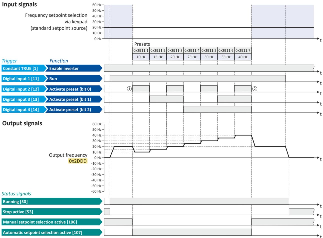
The status signals can be assigned to digital outputs. ▶ [Configure digital outputs](#) 292
