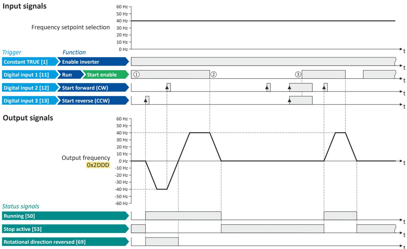
The status signals can be assigned to digital outputs. [▶ Configure digital outputs](#) 292
