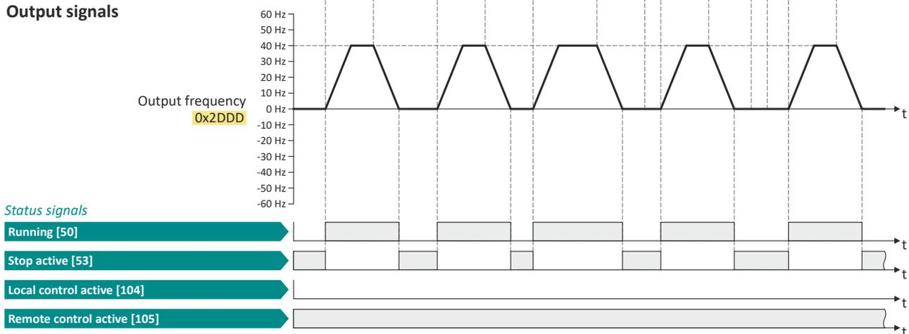
The status signals can be assigned to digital outputs. [▶ Configure digital outputs](#) 292
