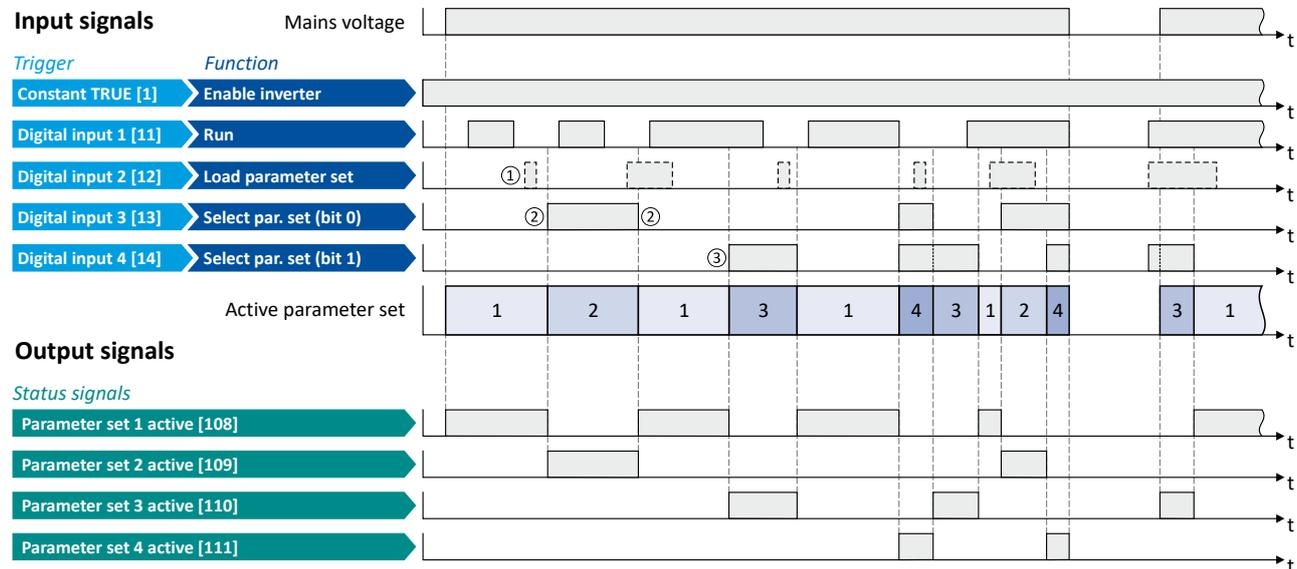
The status signals can be assigned to digital outputs. ▶ [Configure digital outputs](#) 292
