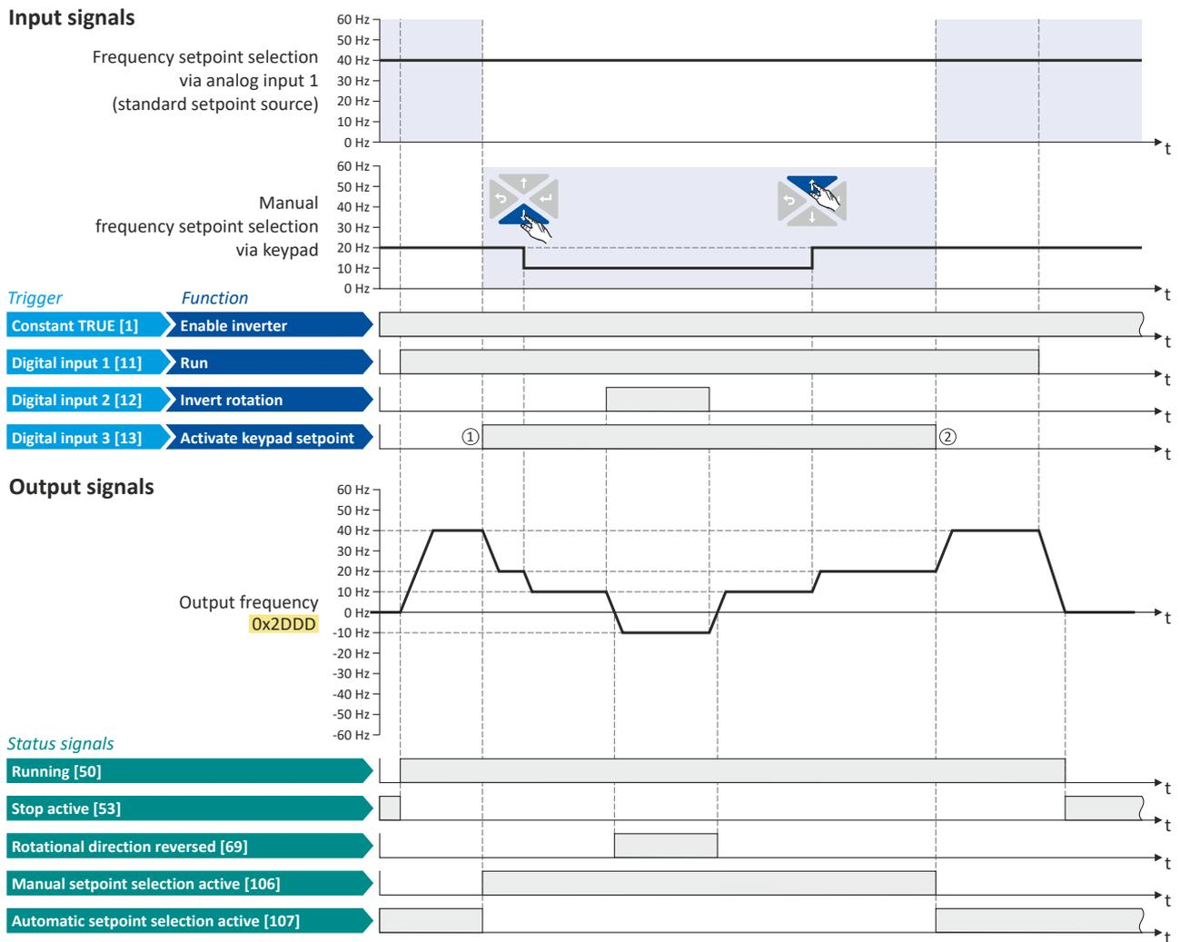
The status signals can be assigned to digital outputs. [▶ Configure digital outputs](#) 292
