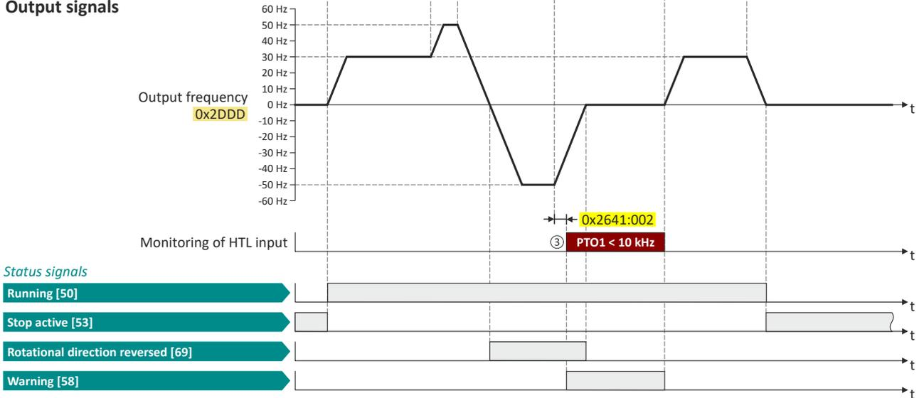
The status signals can be assigned to digital outputs. ▶ [Configure digital outputs](#) 292
