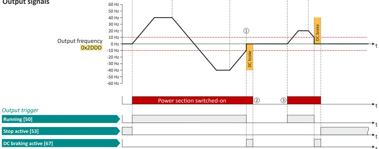
The status signals can be assigned to digital outputs. [▶ Configure digital outputs](#) 292
