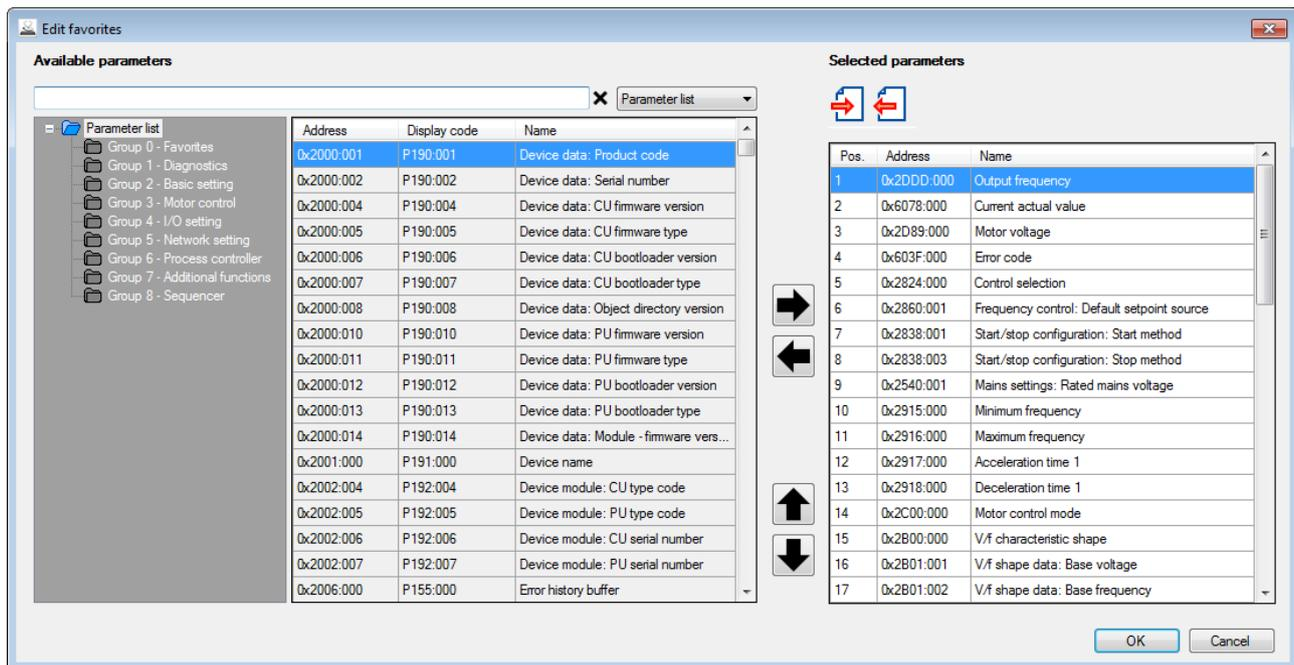
The default favorites can be modified using the keypad or via the network with the following parameters:
