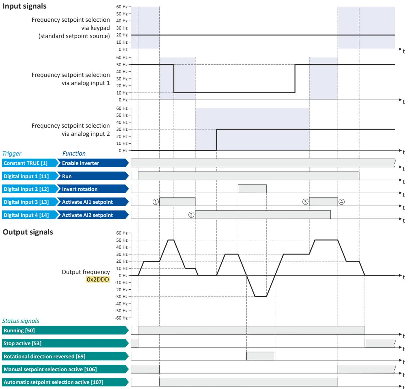
The status signals can be assigned to digital outputs. ▶ [Configure digital outputs](#) 292
