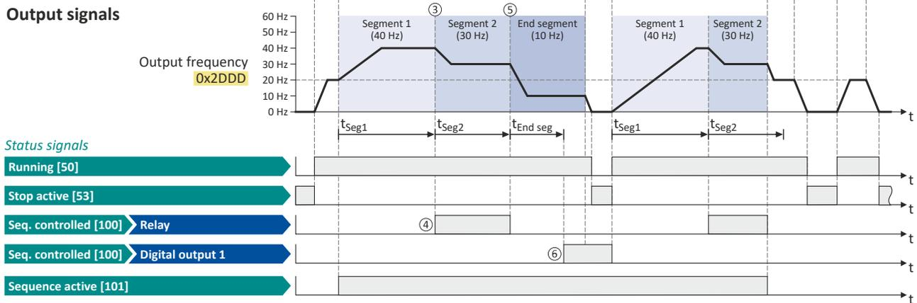
The status signals can be assigned to digital outputs. ▶ [Configure digital outputs](#) 292
