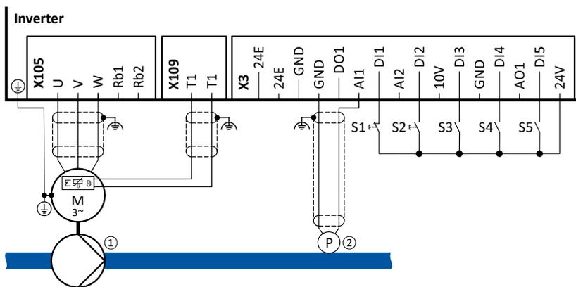
The digital inputs can be used to activate functions of the process controller. The specific assignment of the digital inputs and type of the contacts (switches or buttons, normally-closed contacts or normally-open contacts) depends on the application.
