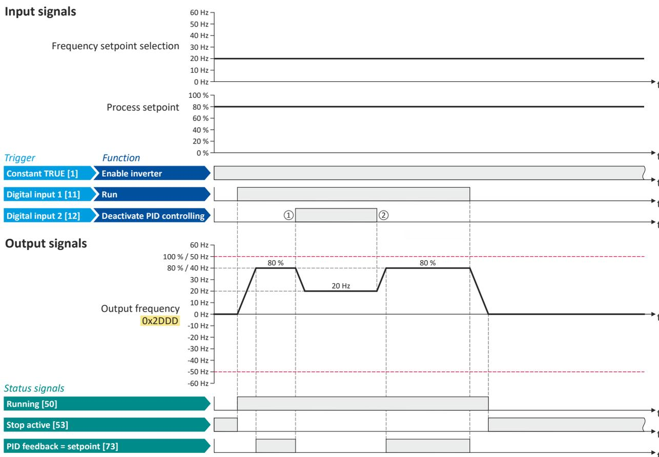
The status signals can be assigned to digital outputs. [▶ Configure digital outputs](#) 292
