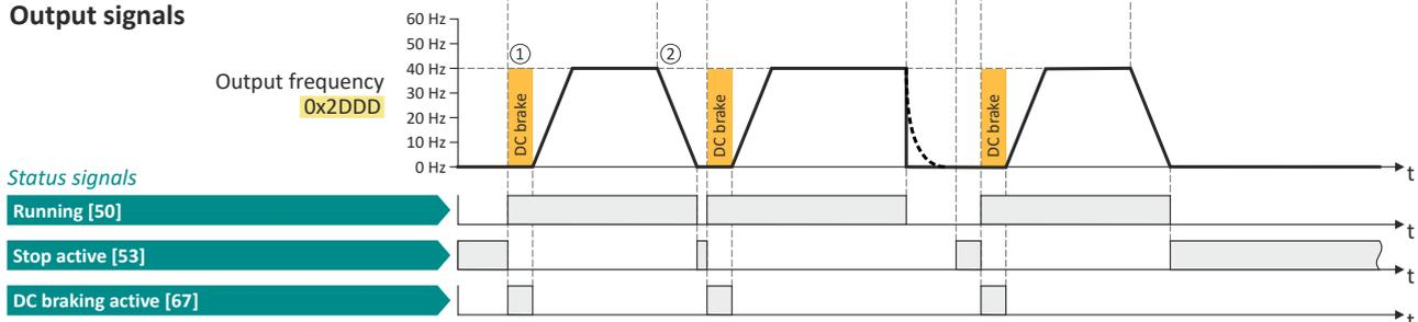
The status signals can be assigned to digital outputs. [▶ Configure digital outputs 292](#)
