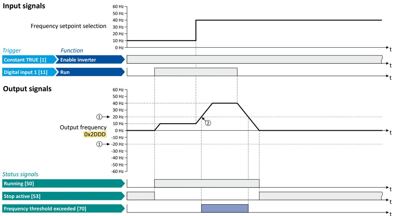
The status signals can be assigned to digital outputs. ▶ [Configure digital outputs](#) 292
