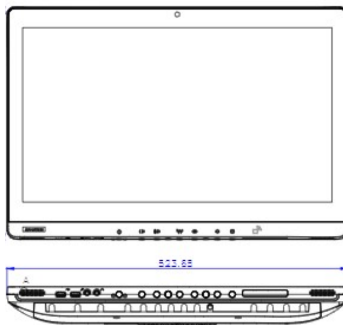
Figure 1.2 Dimensions of the POC-624-12 Series Device with Smart Card Reader
