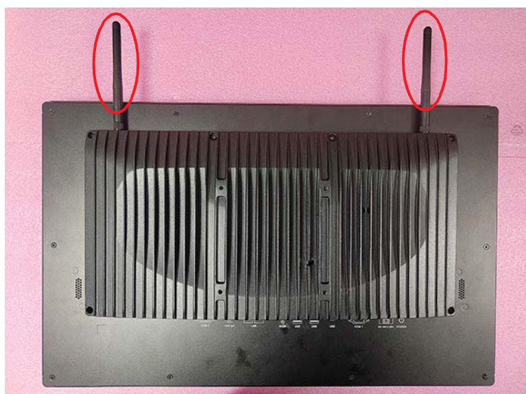
Figure 2.15 Attach the Wi-Fi Antennae
