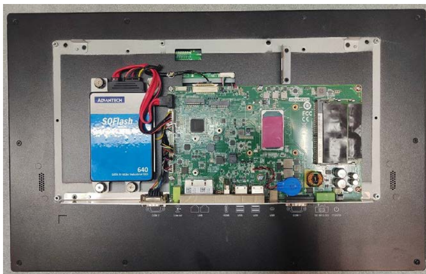
Figure 2.10 SATA SSD Connected to the Motherboard
