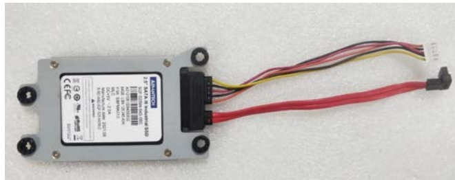
Figure 2.9 Secure the SATA SSD with Screws
