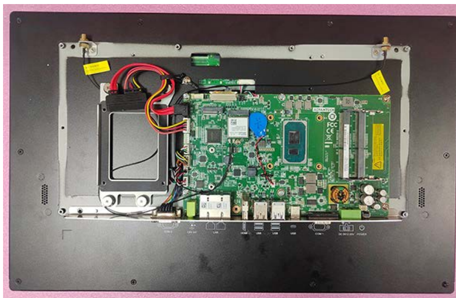
Figure 2.14 Assemble the Wi-Fi Card
