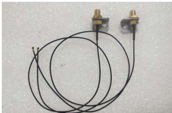
Figure 2.13 Assemble the Brackets to the Antenna Cables
